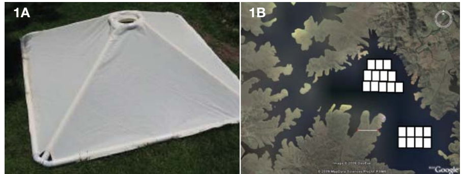
Fig 1A. Modular EMCs comprise a floating framework covered with a reflective fabric. Figure 1B. An image of part of Wivenhoe dam with white rectangles superimposed to represent the appearance of twenty reflective pods, each pod (0.5 km x 0.5 km) comprising 800 EMCs. The twenty pods shown would yield about 10 GL/yr by reducing evaporation.
