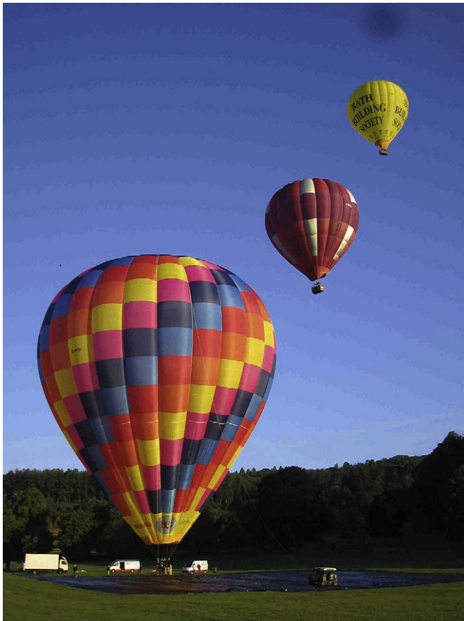
Fig. 1. The envelope of a Cameron Z-1600 hot air balloon. This balloon develops about 6 tonnes lift when charged with air at 60 °C.
